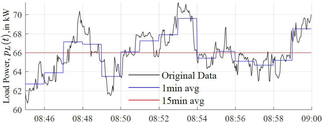
Figure 3 Comparison of different aggregation profile intervals<sup>5</sup>
