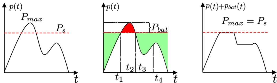
Figure 1 Peak Shaving explained: (f.l.t.r.) a) Before Peak shaving: The Maximum Peak ( $P_{max}$ ) exceeds the peak limit ( $P_s$ ), leading b): Battery action. This peak will be capped by the operation of the BESS. c) After the action of the BESS the peak is shaved and the load profile does not exceed the peak shaving limit.
