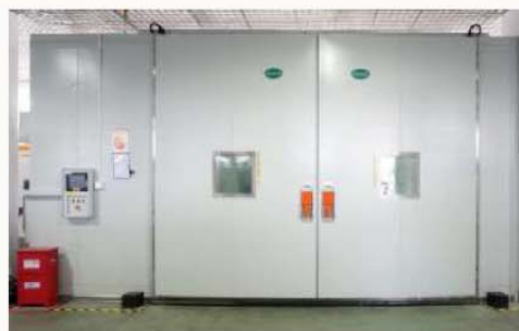
Alternating temperature humidity test
